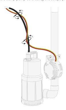
4) Plug the pump power plug into the AC PowerSwitch.
