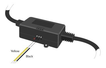
**7)** Secure the AC PowerSwitch so the connected wires are stable. Then plug in the AC PowerSwitch to the AC receptacle.
