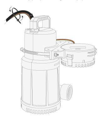
**3b)** Secure all three BG-SP sensor wires along the AC power cable sump pump cord using the straps provided.
